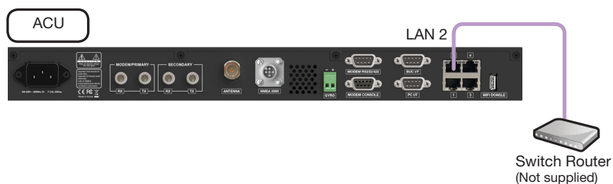
Figure: ACU to Switch Router Cable Connection
