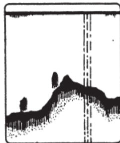
Interference from electrical equipment
