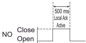
Active interval of Local ACK signal is 500 ±5 msec.
