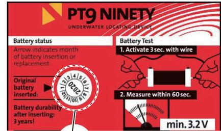
Record this date (date of inserting the internal battery) + three years.
