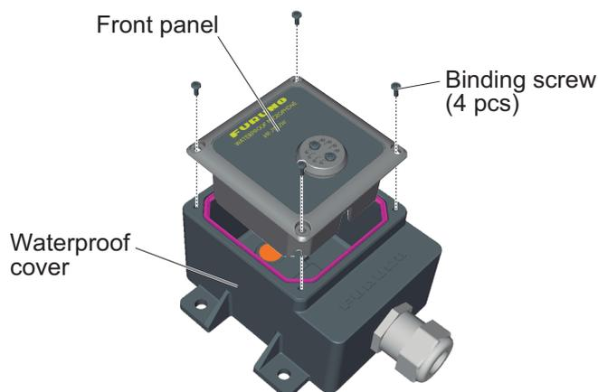
2. Fasten the waterproof cover to the mounting location with four self-tapping screws (supplied).
