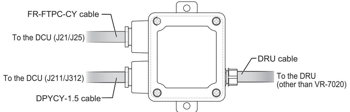
1. Remove four screws to remove the cover from the junction box.
