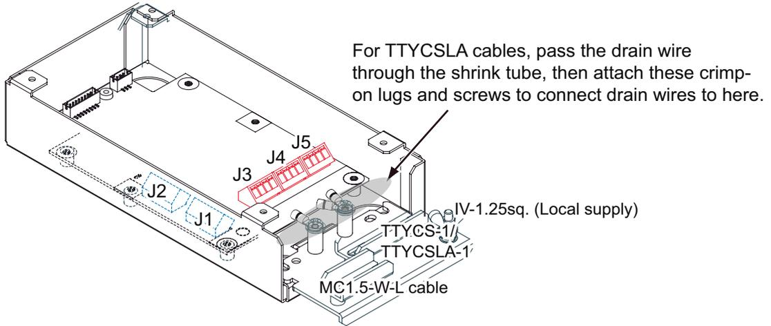
Note: Fasten the cable shield with the cable clamp.
