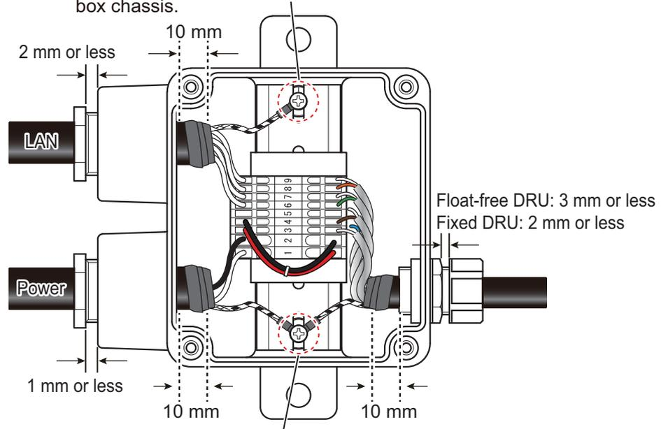
Secure the shield (drain wire) of the DRU cable and the shield (armor) of the DPYCY-1.5 cable to the junction box chassis.
