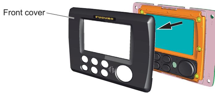
7. Set the unit to the mounting hole, then fix the unit with four self-tapping screws (supplied).
