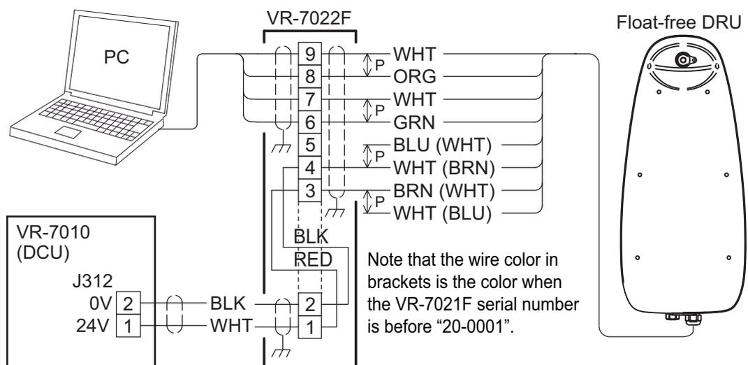
4. Turn the DCU on to supply the power to the float-free DRU.
