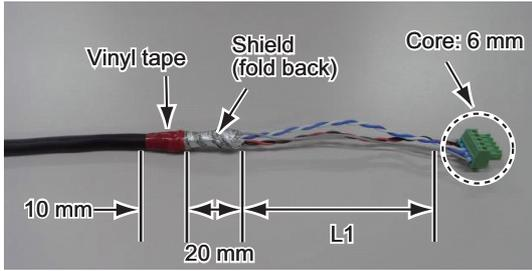
Fabrication of MPYC-12 cable (MC-3020D)
