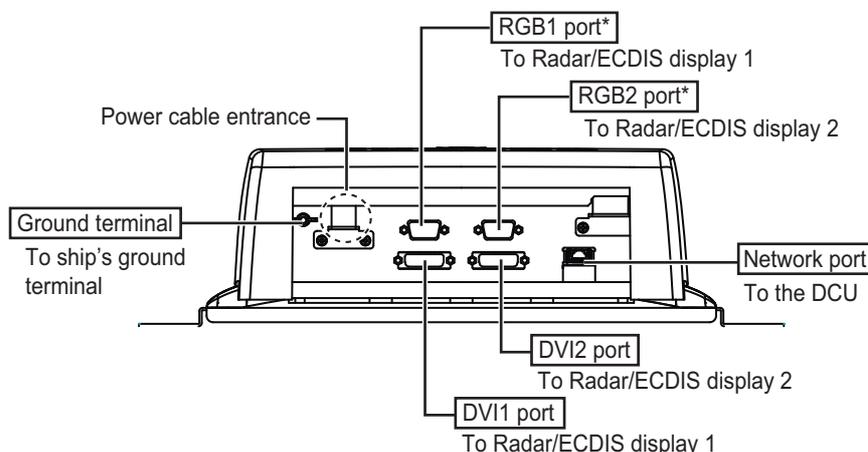
The video LAN converter has two input channels for DVI-D and two input channels for RGB\*. The combinations of input channels shown below are available. Set the input channels for the video LAN converter, using the VDR Maintenance Viewer program. For how to set, see the instruction manual of the VDR Maintenance Viewer (OME-44852).
