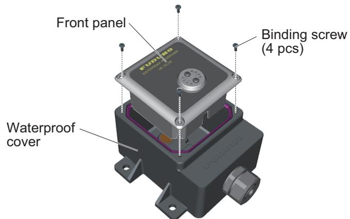
2. Fasten the waterproof cover to the mounting location with four self-tapping screws (supplied).
