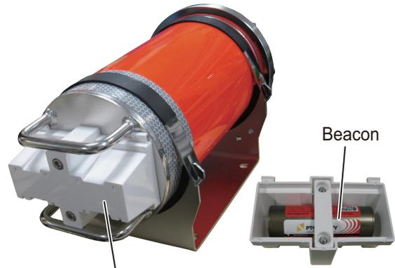
The beacon is attached to the rear side of this cover. Unfasten two screws to remove the cover and expose the beacon.
