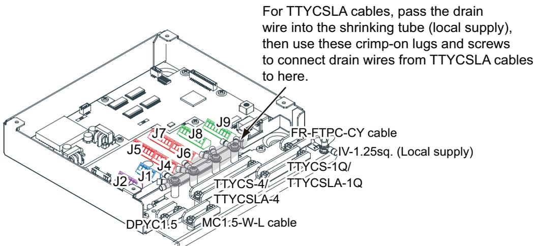
**Note:** Fasten the cable shield with the cable clamp.
