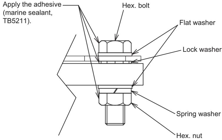
**Hull Grounding Technique**
