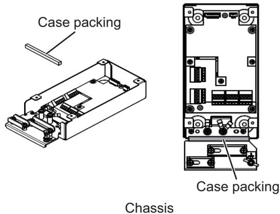
3. Attach the cover to the MC-3010A/3020D chassis.
