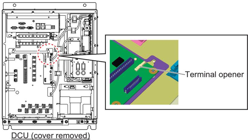
You can use the slotted head screwdriver instead of the terminal opener.
