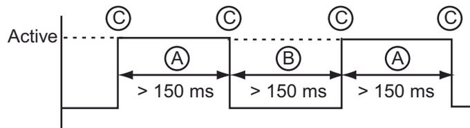
Active interval (A) and (B) of Remote ACK signal shall be more than 150 msec.
