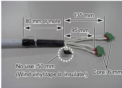
How to connect wires to the WAGO connector
