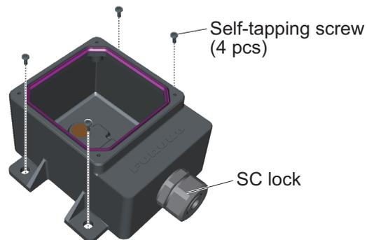
3. Remove the nut and sealing insert from the SC lock.
