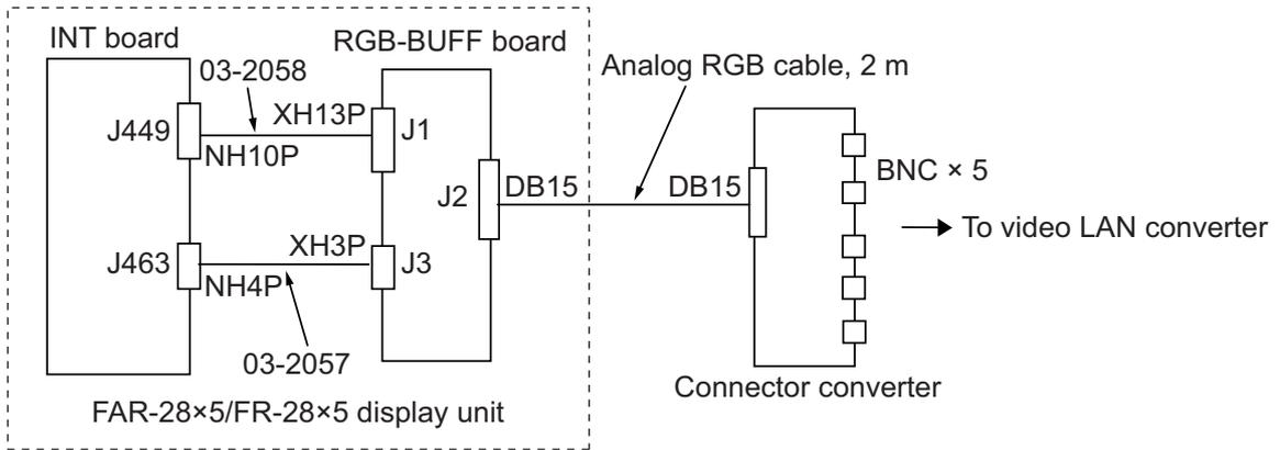
The figure below shows how to mount CPA/TCPA board together with RGB-BUFF board in the FAR-28x5/FR-28x5 series radar. The VDA/INT chassis should be new type, 03-133-1127-4. The CPA/TCPA is powered from #6 (12 V) and #8 (GND) of the power terminal block DTB-2. The J463 port on the INT board is used for the RGB-BUFF board.
