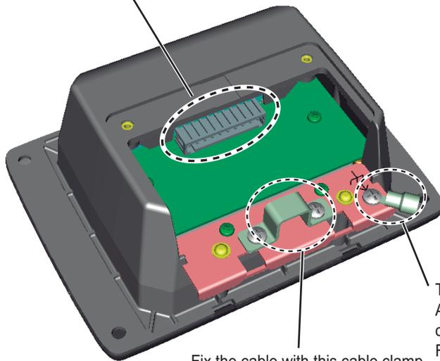
Fix the cable with this cable clamp.
