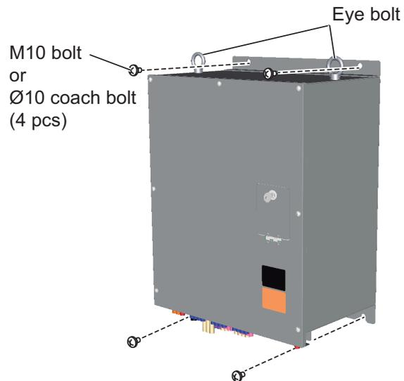
2. Two eye bolts are attached at the top of the unit to hoist the unit onboard. Remove them after the installation.
