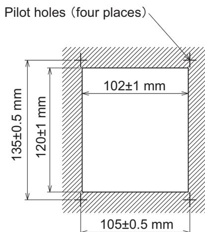
3. Fasten the front fixing panel (option) to the mounting hole with four self-tapping screws ( $\phi 4 \times 16$ ).
