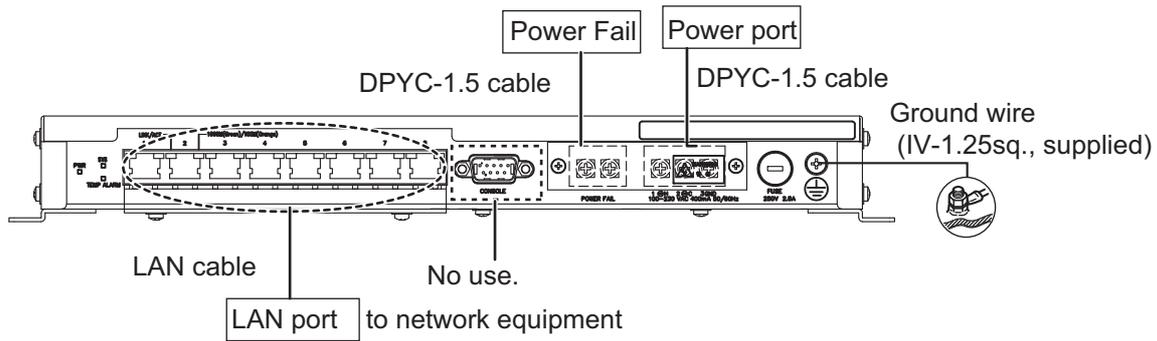
Attach the LAN port cap (supplied) to the unused connector holes to provide waterproofing standard IPX2.
