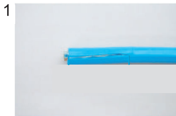
1 Expose inner vinyl sheath.
