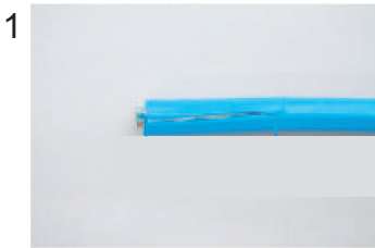
Expose inner vinyl sheath.
