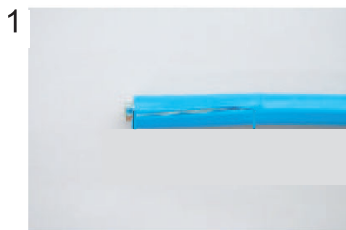
1 Expose inner vinyl sheath.
