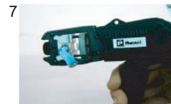
7 Using the special crimping tool MPT5-8 (PANDUIT CORP.), crimp the modular plug. Finally, check the plug visually.
