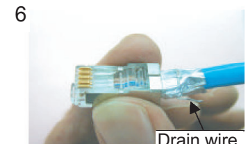
6 Insert the cable into the modular plug so that the folded part of the shield enters the modular plug. The drain wire must be on the tab side of the jack.
