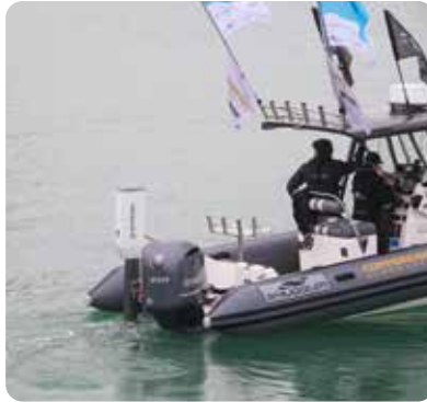
THE WASSP W3P BRACKET MOUNT ALLOWS FOR SIMPLE AND FAST RETROFIT INSTALLATION ON A WIDE RANGE OF TENDER VESSELS.
