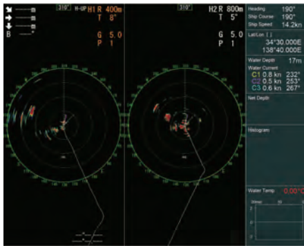
Horizontal scan 1 Horizontal scan 2 Range: 150 m Range: 300 m Tilt: 45 degrees Tilt: 20 degrees Gain: 5.0 Gain: 5.0
